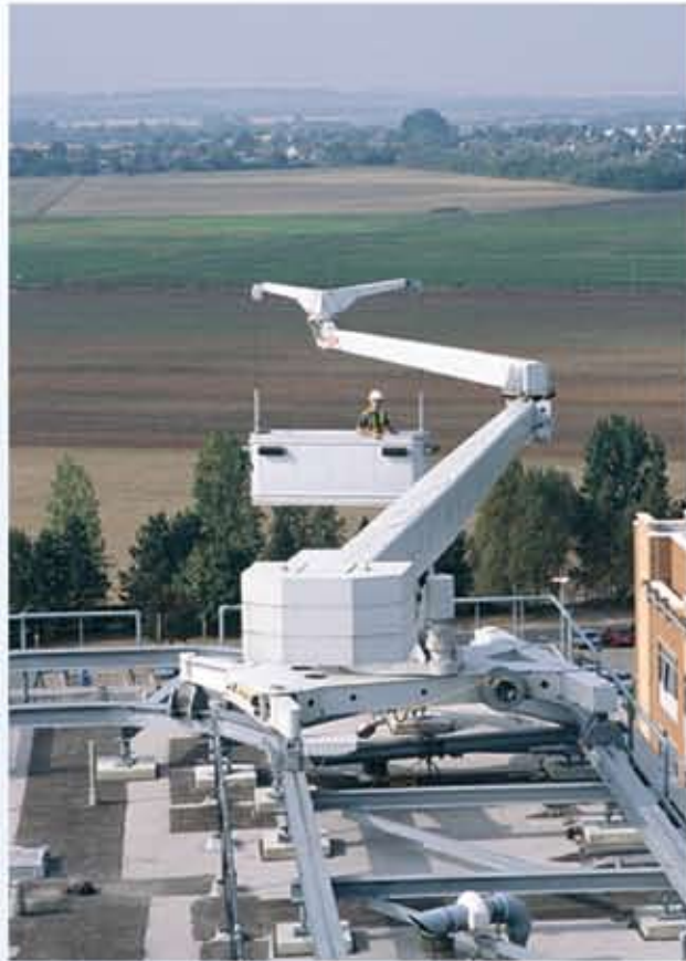
Type 6.1, track-based with horizontal slewing articulated jib
