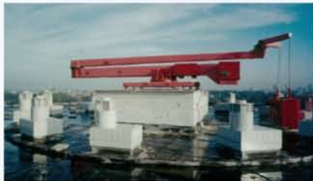
Type 6.4, stationary with horizontal slewing articulated jib for minimal parking position on a circular building
