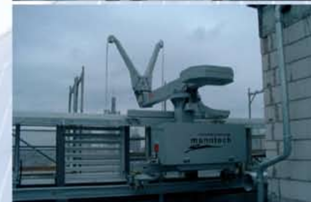
Type 4.2 low profile design with high V-head
