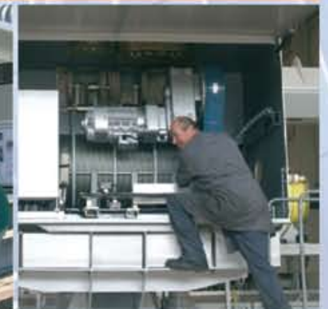
High-performance hoist unit, approx. 4,000 kg lifting capacity
