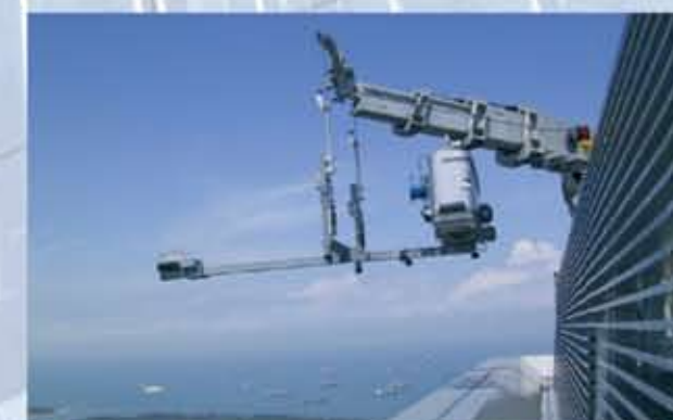
Various satellite cradle solutions for reaching recesses in building
