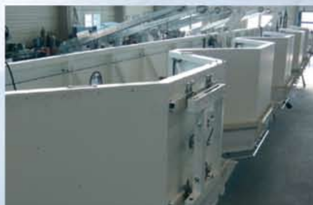
Customised cradle (platform) 15 m long for replacing large façade elements
