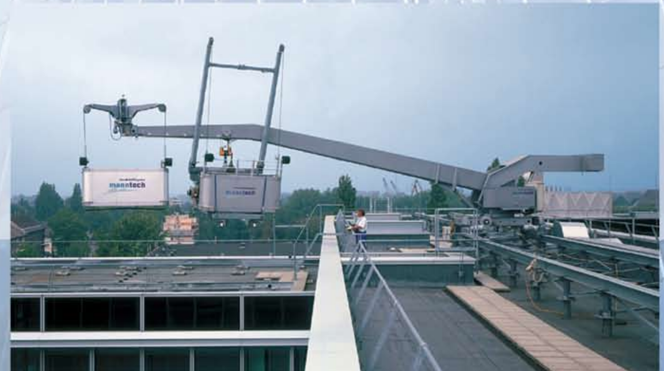
Type 6.1, track-based with fixed luffing jib and mechanism (load-bearing hoist) for transportation of a Type 1.1 machine to various parts of the building
