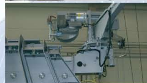
Auxiliary hoist to transport glass panels and façade elements outside the cradle—movable or fixed installation
