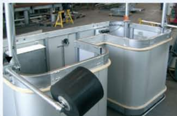
Customised cradle (platform) solutions to fit building requirements
